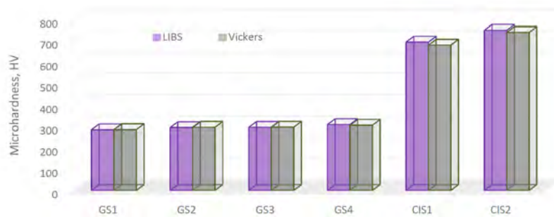
Fig. 1: Comparison of LIBS and Vickers method. Determination of microhardness of glass (GS1, GS2, GS, GS4) and cast iron (CIS1, CIS2) samples using LIBS and standard Vickers method.
