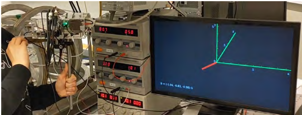
Fig. 3: A handheld prototype device for measuring the direction and magnitude of a magnetic field using a diamond with NV centers.
