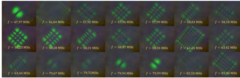
Fig. 1: Various TEM modes for 532 nm light while FP cavity is locked on 1064 nm TEM 00 mode. Yellow labeled numbers correspond to the AOM frequencies used to get represented TEM mode [1]
